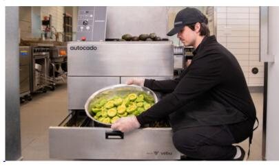
Vebu's signature robotic product is the Autocado, the pioneering avocado-processing robot which eliminates the need for restaurant workers to cut, core and scoop avocados to prepare guacamole. The Autocado allows employees to load up to 25 pounds of avocados into the device and walk away to focus on serving customers and preparing other items. It is now in pilot testing in Chipotle's Huntington Beach, Calif. restaurant.
